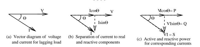
Figure 1: Vector Diagram for an Inductive load
