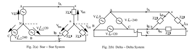
Figure 2: Schematic configuration of star – delta supply and load system
