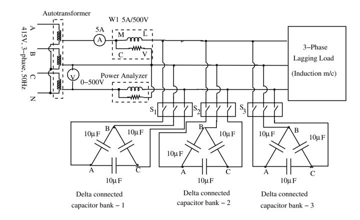
Fig.6 Circuit diagram for Power factor improvement
