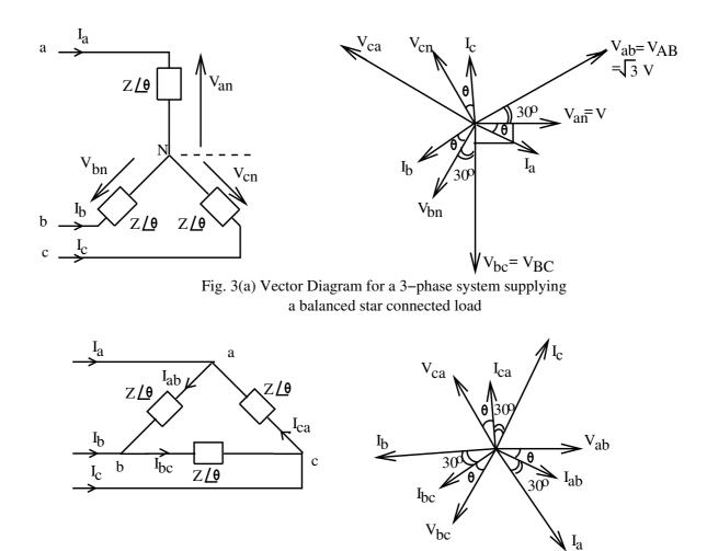
Fig. 3(b) Vector Diagram for a 3–phase system supplying a balanced delta connected load
